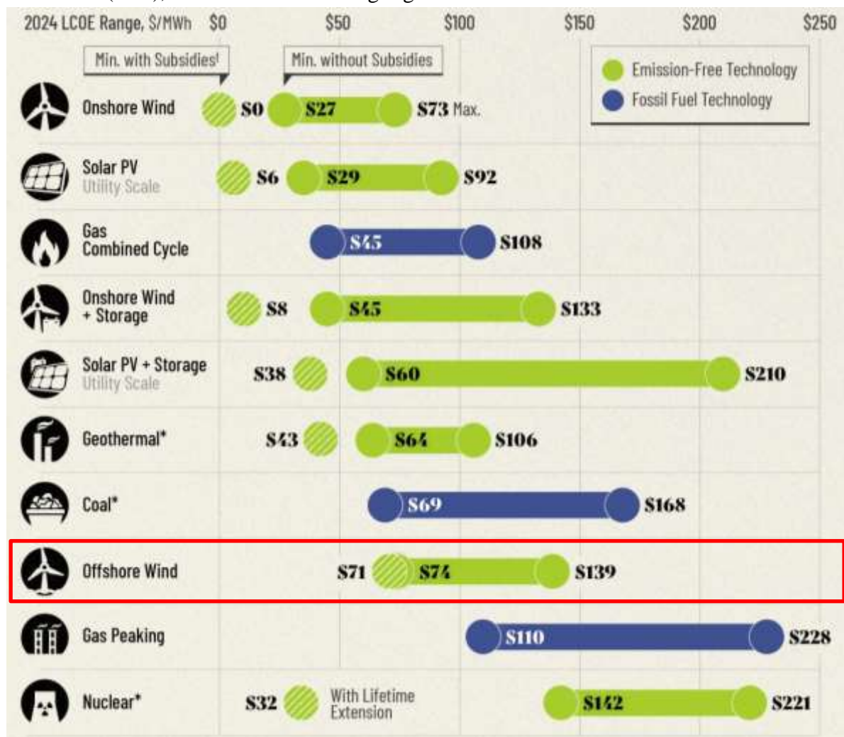
Figure 5. Estimated costs of electricity today, including from renewable sources (green) and fossil fuels (blue), with offshore wind highlighted in red. 44
