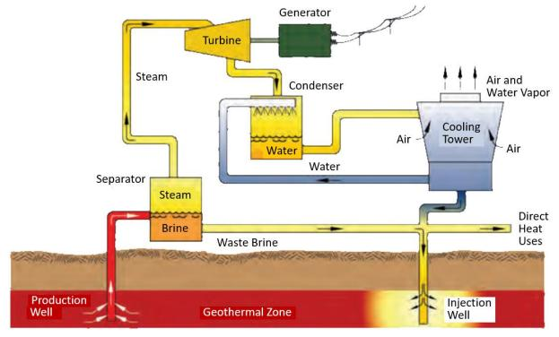
Figure 7: Flash Steam Geothermal Power Plant
